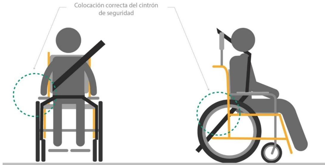
Para mayores detalles de las especificaciones se pueden consultar las normas *ISO 10542-1 Technical systems and aids for disabled or handicapped person – Wheelchair tiedown and occupant-restraint systems – Part 1: Requirements and test methods for all systems*, o la *ISO 7176-19 Wheelchairs – Part 19: Wheeled mobility devices for use as seats in motor vehicles*.
